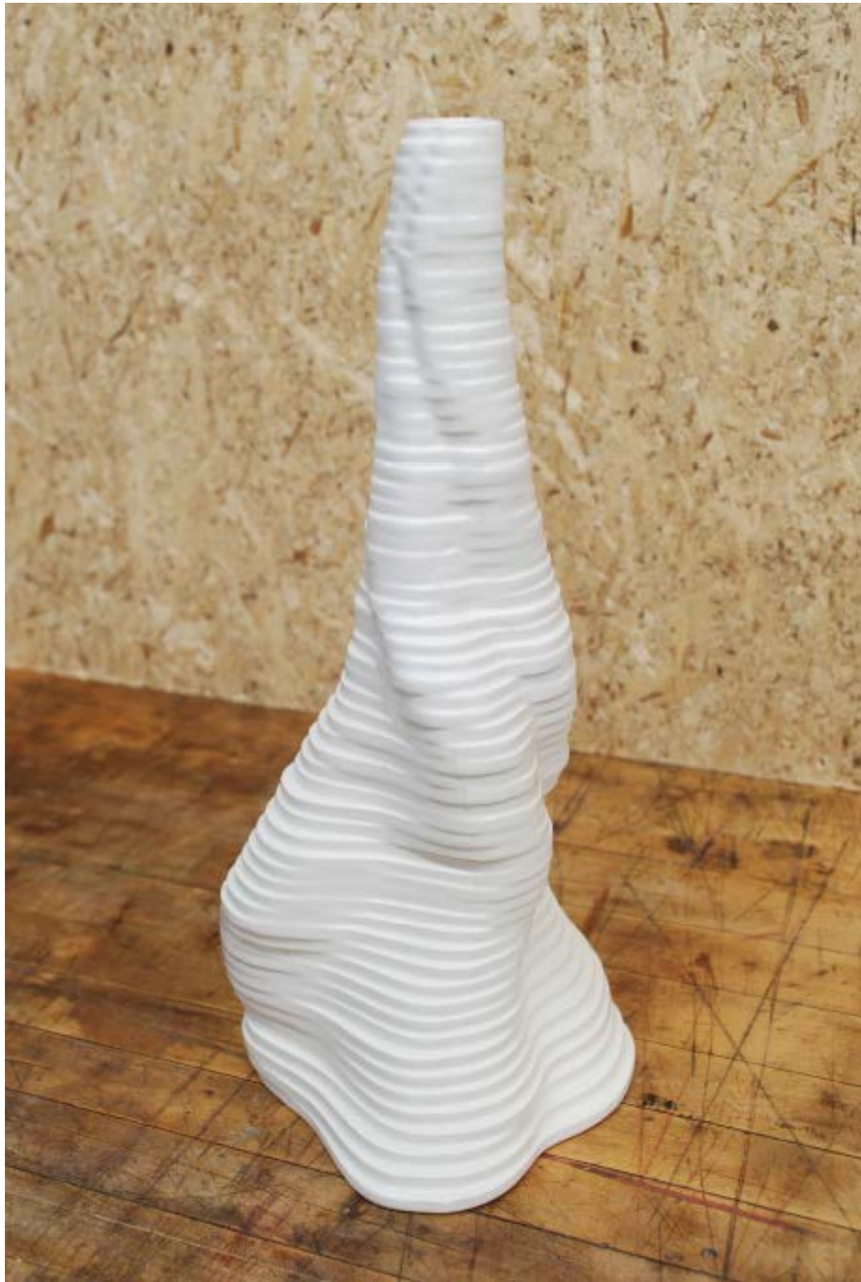
Ceramics: Slipcast from Molds Derived from Stacked Laser Cut Acrylic and CNC Routed MDF
