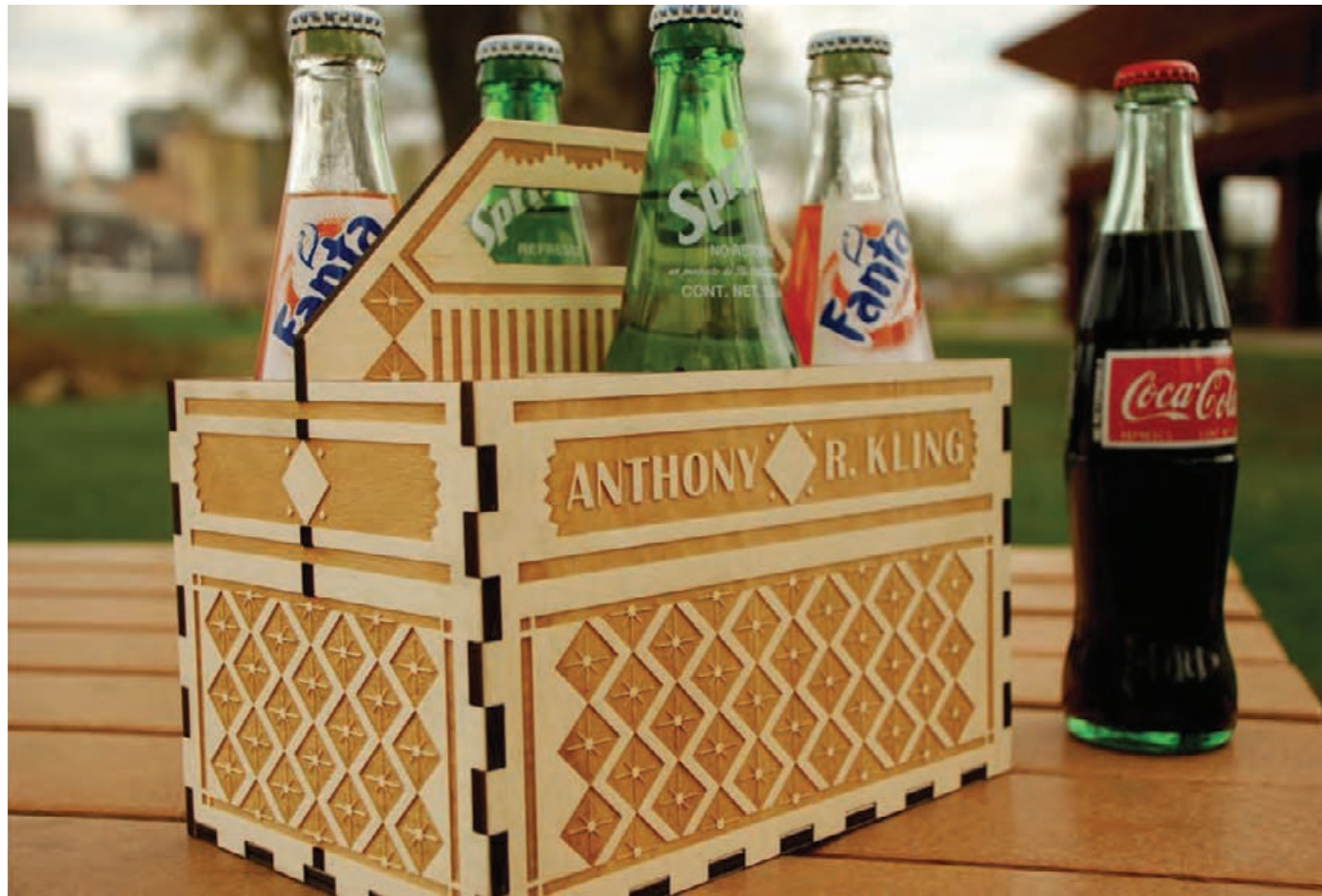
Custom Six Pack: Features Precision Laser Cut Wood Joinery and Laser Etched Surface Design
