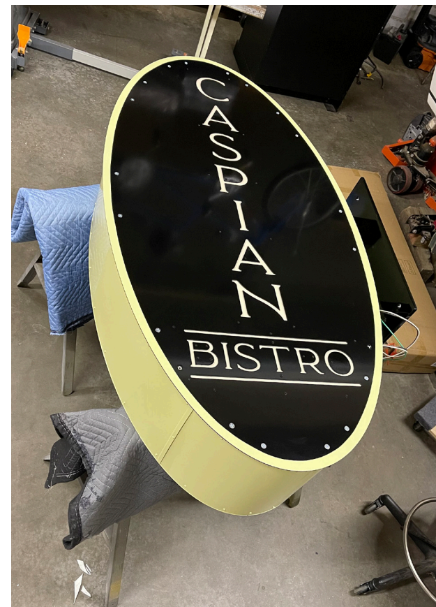
ARK: Caspian Bistro Custom Sign Featuring Retrofitting Old Sign Frame, Fabricating New Face and Return Panels and Installing LED Mounting Panels
